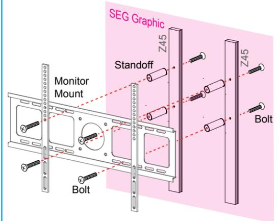
Attach standoffs to vertical extrusions, using bolts then attach monitor mount to standoffs, using bolts.
