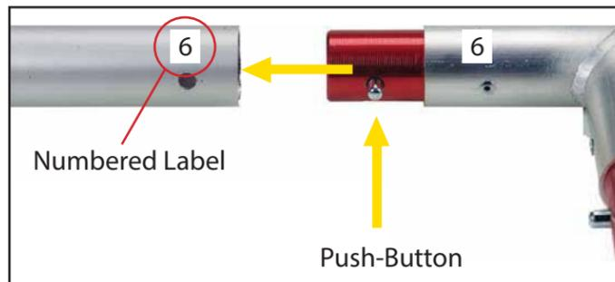
Connections are made by holding the button down and sliding the red tube into opposing tube until button locks into the hole. To disassemble, push button and pull or twist extrusions apart.
